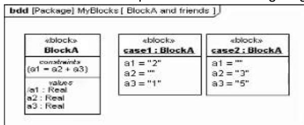
The modeler has set all shown values as inputs and next intends to solve the model that is, to calculate the outputs. Assume nothing relevant has been left out.
